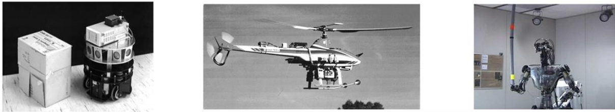
Figure 2 – Robots with behaviors that were reinforcement learned (From left: OBELIX, autonomous helicopter, Sarcos humanoid DB) (Kober, 2013)
